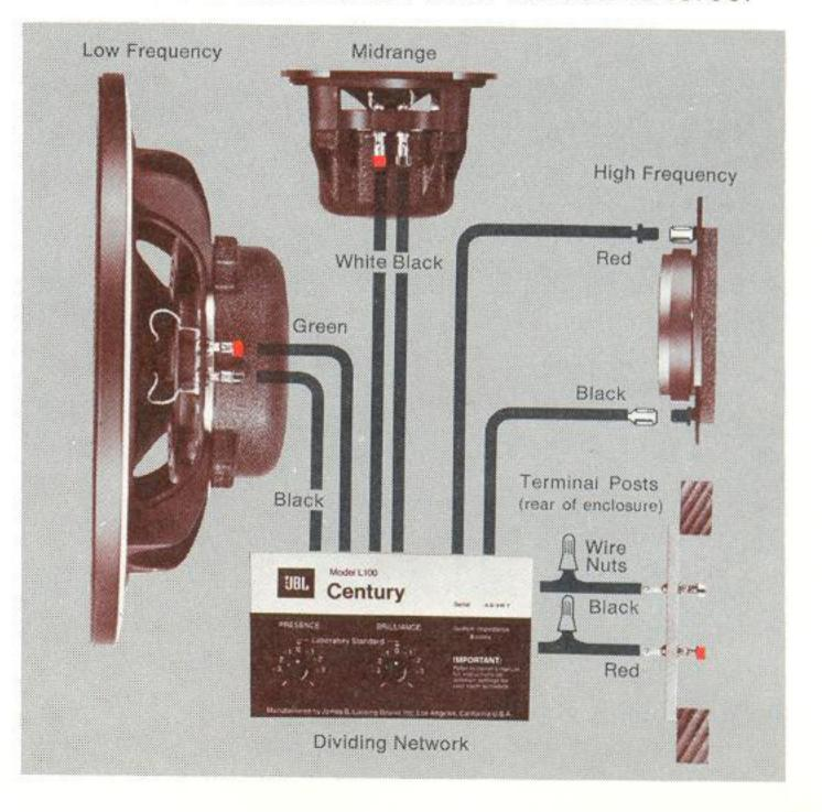
Wiring—When reconnecting the wire leads between the dividing network and the components, observe the polarity shown at the left.
