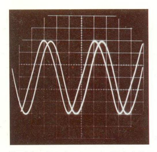
Sustained performance at this intensity would not be encountered during normal use. A 50 Watt RMS test signal is far more difficult for a speaker to reproduce than its rated capacity of 50 Watts program material, specially in the lowest register of the audio spectrum. Nevertheless, it can be seen that the L100 produces a virtually perfect replica of the input signal.
